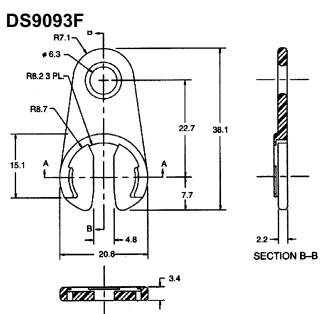
SECTION A-A All dimensions are in millimeters.
