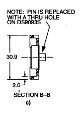
The DS9093S and DS9093P allow the user to permanently attach an <u>i</u>Button to an object with one or two screws, rivets, etc. The plastic plate is designed with an inset that accommodates the flange of the F5 package and allows for flush mounting. A protective wall is provided along the sides of the plate to reduce incidental damage to the <u>i</u>Button.
